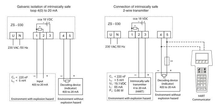
Voltage drop for device without HART signal transparency < 230 mV / 21 mA.
